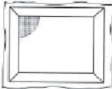
Two corners of the frame are stapled taking care that the staples are at 45° and with a spacing of 5 to 10 mm. between each staple.
