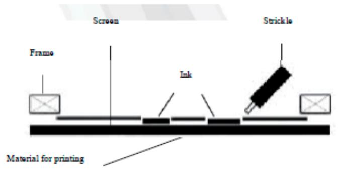
In screen printing a cliché or stencil can be obtained through the following methods:
