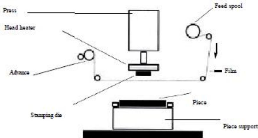
In special cases, dies can be manufactured of silicone rubber, specifically provided that the surface is flat or when for any inaccuracies in the production of the pieces the differences have to be compensated.
