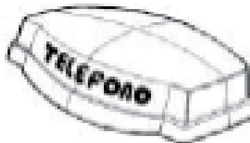
There are pieces that will need to be printed after thermoforming as is the case of lighted ads or others where the bas-relief is the printing area. There are two methods to do this type of printing:
