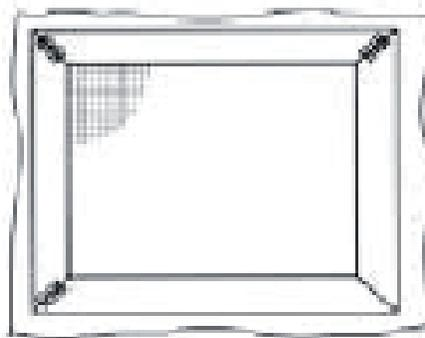
Staples are placed at 45° every 10 to 15 mm. on either side (this is done with the object of the staple not tear the mesh).
