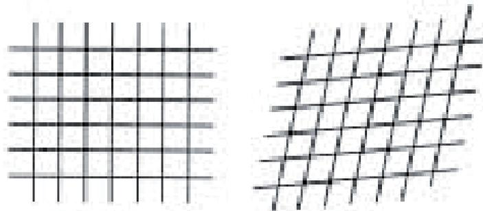
Uneven tension causes the threads of the mesh to deform causing uneven printing.
