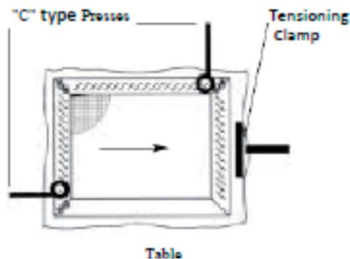
The last side is tensed, stapled and the overlap cut with a cutter and lastly a wood varnish or lacquer is applied on all staples with a brush.
