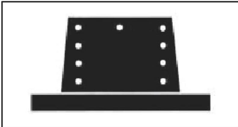
4. When the dimensions of the formed piece are critical, molds must be constructed in larger sizes to compensate for shrinkage of the material. Shrinkage to be expected from the molding temperature to ambient temperature is 1% maximum.
