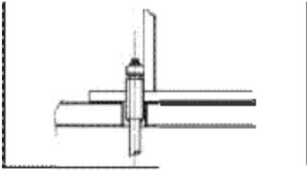
Cutting with router, straight bit and cutting guide
