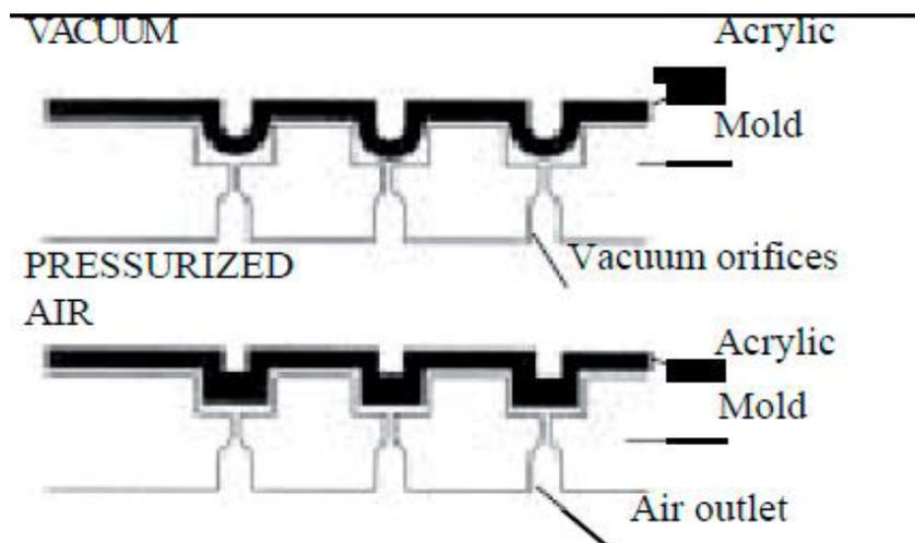
The mold, when required, must have holes for ventilation of trapped air and thus prevent wrinkles or deficient formings.
