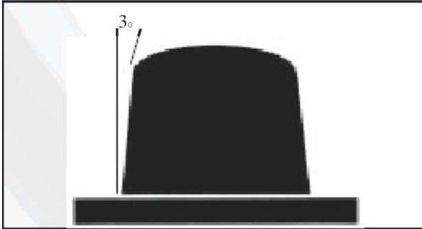
7. It is advisable to round the corners, since vertex forming accumulates internal stresses. The strength of the piece will be greater by designing rounded sides, corners and edges.
