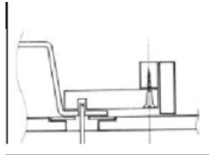
Cutting with router and biscuit cutter or abrasive disc on the outside
