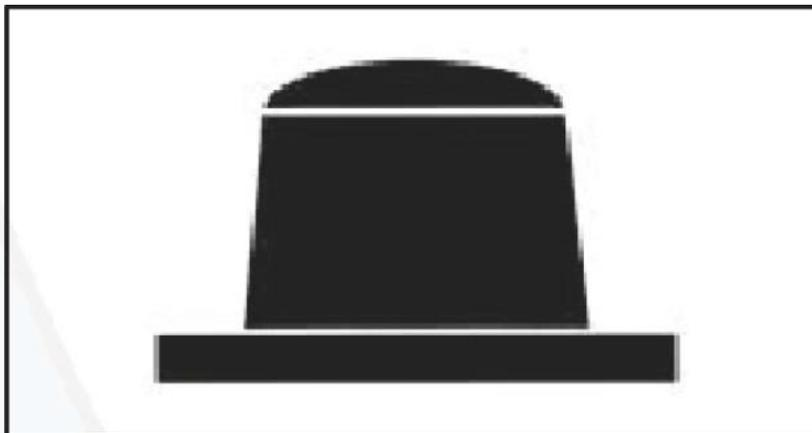
6. Pieces with walls at  $90^\circ$  cannot be obtained, the mold should have an exit angle of at least  $3^\circ$
