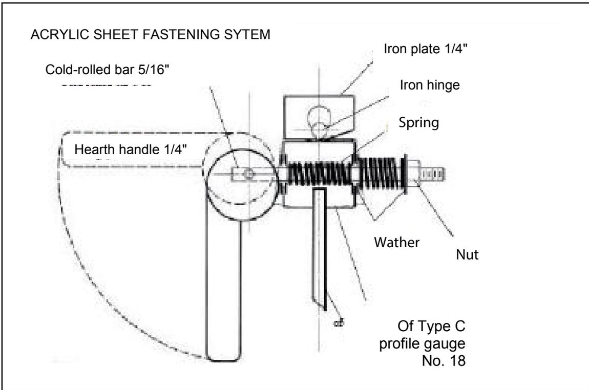
FRONTAL VIEW AND DETAILS OF THE OVEN DOOR AND SLIDING SYSTEM Fastening to the
