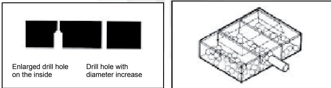
Another function of the mold is to contribute together with the frame to stabilize the position of the sheet and support a good seal around the entire periphery of the mold, in some cases it is convenient to make a channel around the piece, precisely on the outside area of the cutting line.
