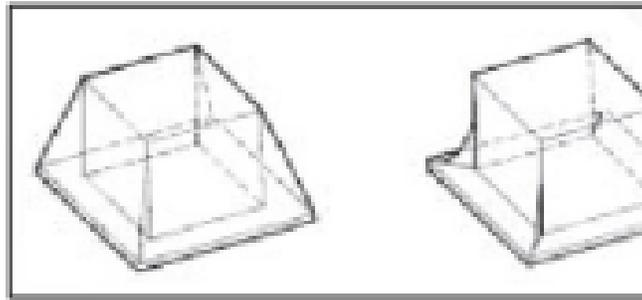
One consideration that should be taken into account is the possibility of wrinkling in a critical area or in the lower part of a male or female mold. If the tempered sheet is unable to shrink from the dimension A to E, the excess material will form wrinkles.
