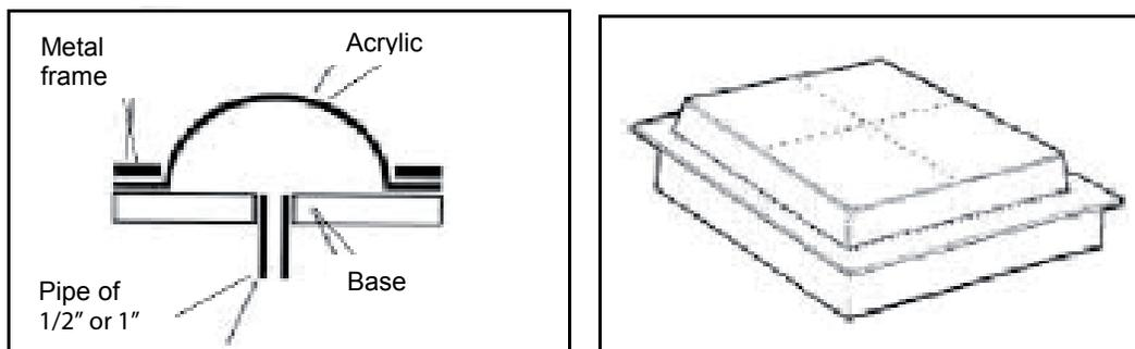
The drawings show the distribution of the vacuum or air pressure drill holes typical of molds for free press forming, male mold and female mold.
