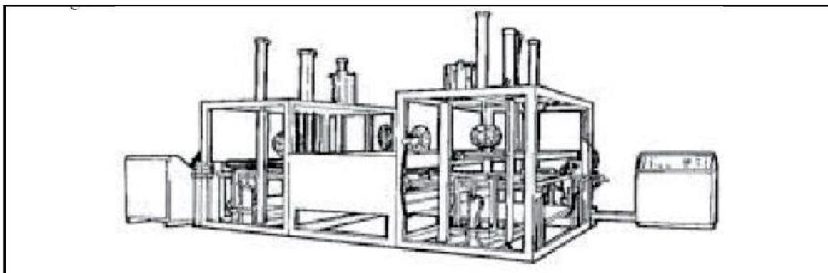
Infrared energy is absorbed by the exposed acrylic surface, quickly reaching temperatures above 180° C to then be transmitted to the center of the material by temperature conduction.
