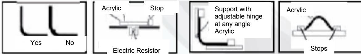
With proper heating clean and bright corners will be obtained.
