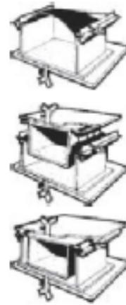
Vacuum forming, female mold and mechanical aid
