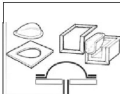
**Forming under vacuum and pressure, female mold** This procedure allows forming in molds pieces whose shape requires more precision than those obtained by vacuum. However the high pressures will cause mold marks on the piece. As high pressures are required, the molds must be made of metal, epoxy resins or other materials that withstand high pressures without deforming. The good finish of the molds is imperative to achieve quality parts.
